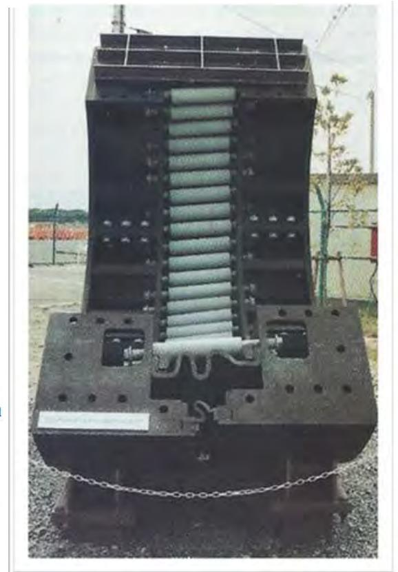
Eight 1,5m wide flexible joint rings are inserted into the primary segmental lining to help the accommodate the settlement and seismic activity
