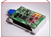
JRC (Joint Research Centre) is developing a diagnostic device for freight trains based on acceleration measurements, which should be integrated within an information network allowing communication between train wagons, locomotive and infrastructure.
