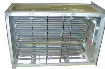
HVAC Passenger car Heating Registers
