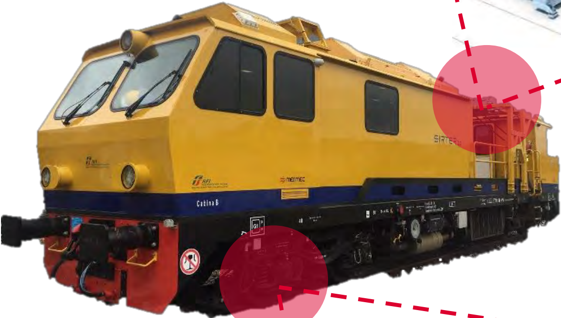
OHL geometry and wear system
