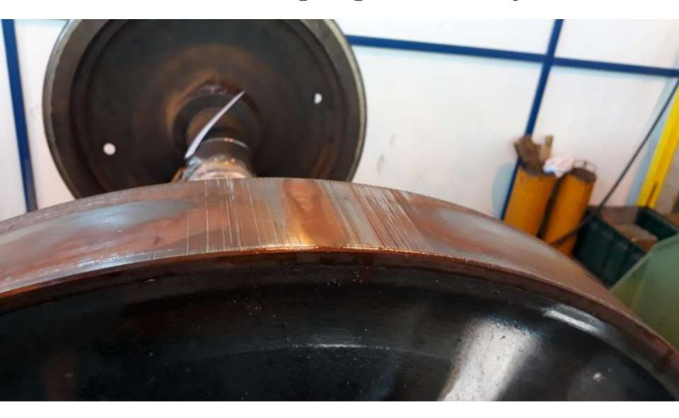
Tyres can be removed by «shrink removal» (no damage!)
