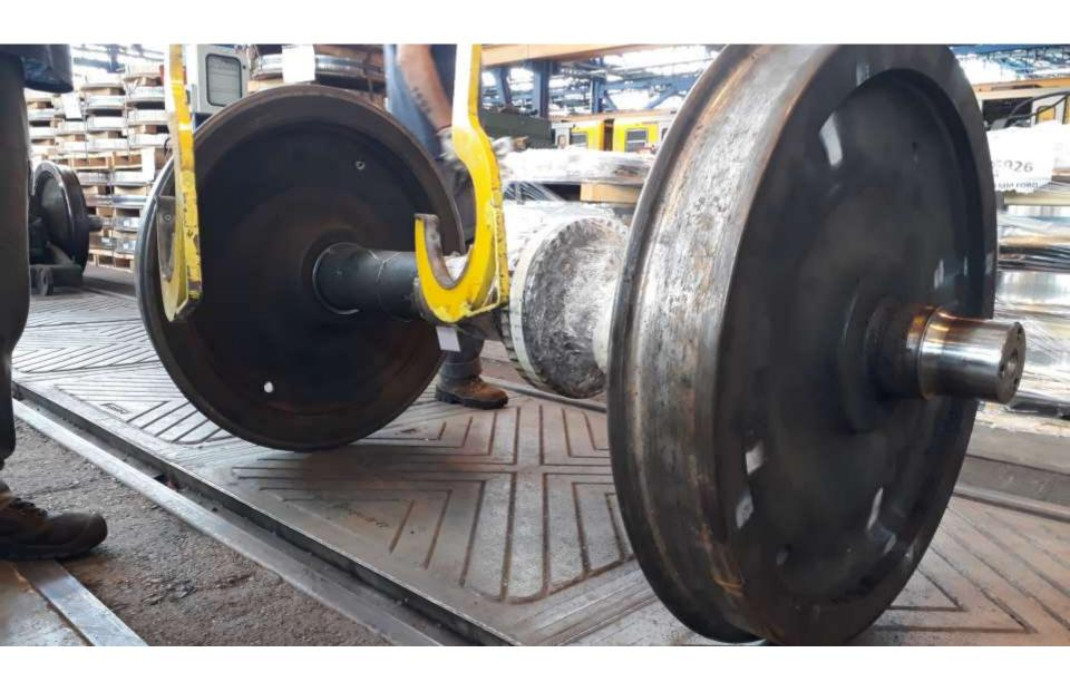
First, the retaining ring must be «turned» on a wheelset lathe to be removed
