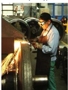
Or, the tyre can be removed by saw cutting + an extractor (damage to wheel centre *very likely*)
