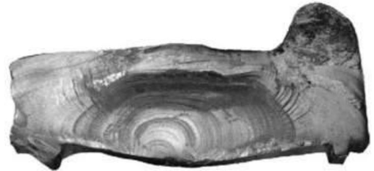
Fig. 4. Fracture surface of the broken wheel tire.
